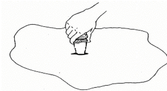
Figure 2. Wood Plug Installation.
